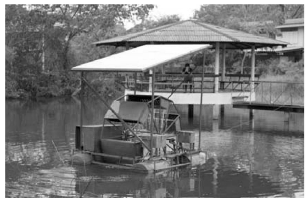
Figure 6 The aeration turbine prototype
